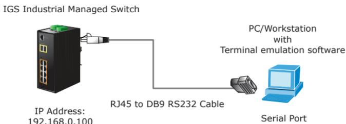
A terminal program is required to make the software connected to the IGS-5225 series Industrial Managed Switch.
